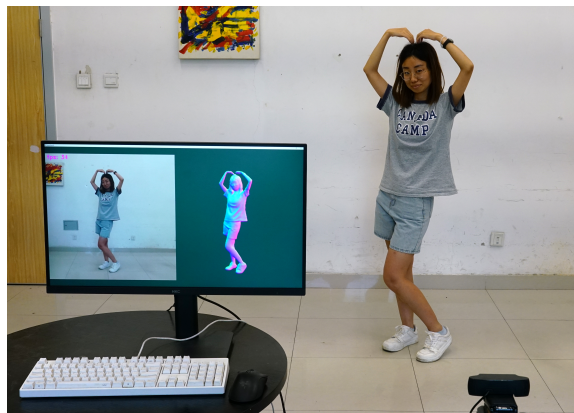
Fig. 13. Our system applied to perform real-time 3D human reconstruction from a single monocular RGB input. Please see the supplement video for the live demonstration.
